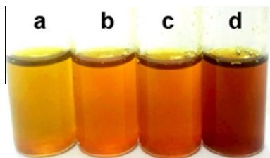
Fig. 1. Colour change in 1% turmeric solution after addition of \text{F}^- ions in DMSO (a) 1% turmeric solution, (b) 1 ppm, (c) 10 ppm, (d) 100 ppm. (For interpretation of the references to colour in this figure legend, the reader is referred to the web version of this article.)
